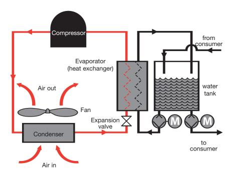
In addition to the above, there are small mobile chillers available which also have a heating capability, e.g. the Tool-Temp TT5000H which cools as a normal chiller but also has 6kW heating power available. These types of machines allow a process to come up to temperature prior to running if, for example the ambient is slightly lower than the running temperature in the winter.
